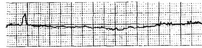
Fig. 7. Fired pellet profile for a 7 g pellet of powder ball milled for 4 h with 0.5 wt% lubricant and pressed at 1\ \text{tonnes cm}^{-2} (Scale: x-axis 1\ \text{mm} = 0.1\ \text{mm} , y-axis 1\ \text{mm} = 2\ \mu\text{m} ).
